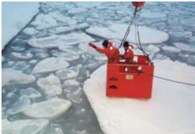
Sampling frazil ice in the water column off East Greenland over the side of a research ship.
